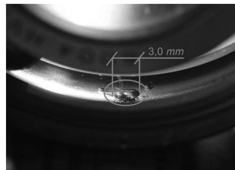
Fig. 7. Vertical axis rotor kit scheme (a) with variable tilt angle  $\gamma$ , piezoelectric transducers X, Y locations at 1<sup>st</sup> and 2<sup>nd</sup> bearings housings and position of outer ring raceway spall (b); photo of the research kit (c); bearing outer ring spall 3 mm diameter (d)
